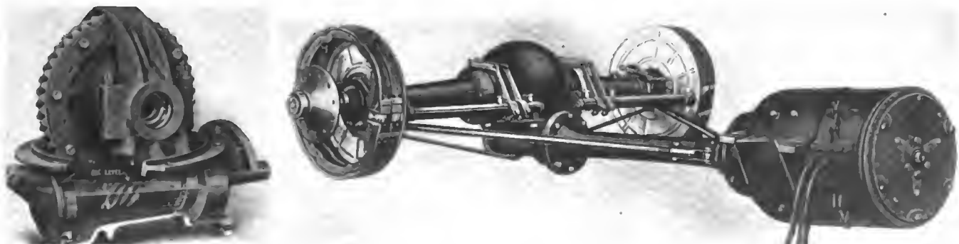
Left—Lancheater-type worm gear used in the Detroit electric. The worm runs in a bath of oil. Right—Drive unit, showing underneath worm and inclosed propeller shaft
